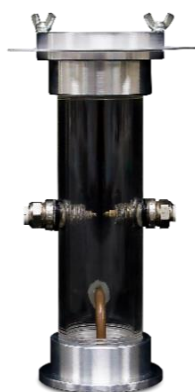
Figure 2: 1.2 L Chamber equipped with two spark plugs.
