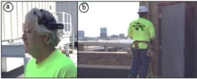
Figure 4. (a) EEG Collection from construction worker the position of wearing the device to detect EEG Signal (b) the integration of EEG device and safety helmet 6.
