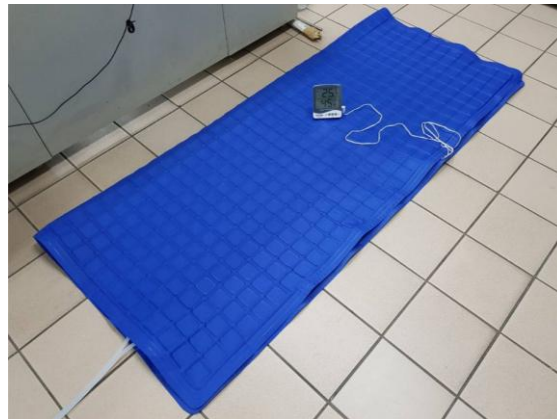
Figure 3. Temperature-controlled cooling blanket prototype components (cooling pad)
