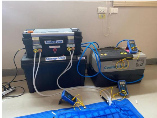
Figure 2. Temperature-controlled cooling blanket prototype components (cooling unit and control unit)
