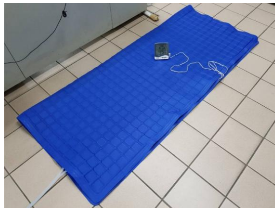
Figure 3. Temperature-controlled cooling blanket prototype components (cooling pad)
